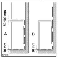
Do not obstruct the space underneath. The back of the cabinet may be placed close to the wall but must not touch it. DO NOT install in places with restricted ventilation. Adjust the level of the appliance by screwing out the adjustable foot, or feet, at the bottom of the cabinet using your fingers.
